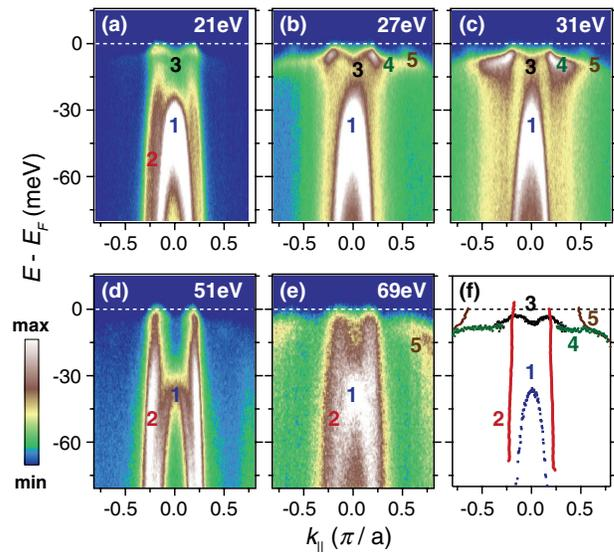
FIG. 1 (color online). (a)–(e) ARPES spectra along the (0, 0) to ( $\pi$ , 0) direction for different excitation energies (noted in the top right of each image) measured at 2 K, deep inside the hidden order (HO) phase. (f) Dispersions of all the different features obtained from fits to corresponding EDC/MDCs.
